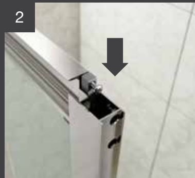
2 Slot the horizontal profile and screws into upright using guide channel until flush.
