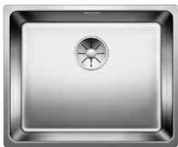
Cut Out Size: 530mm x 430mm x 15mm corner radii Bowl Depth: 190mm Cabinet Size: 600mm
