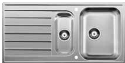
Cut Out Size: 982mm x 482mm x 15mm corner radii Bowl Depth: 155/130mm Cabinet Size: 600mm
