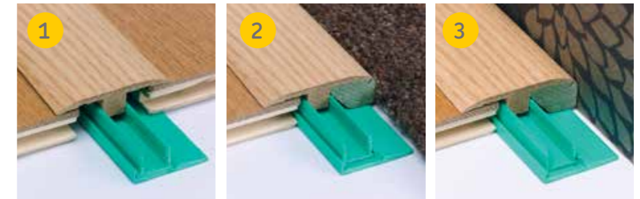
1 Expansion Profile to cover expansion gaps between two adjacent flooring products of the same height. 2 Adaptor Profile for use when finishing between two adjoining floor coverings where the adjacent floor covering is of a lower height e.g. carpets or vinyl. 3 Edge Profile to finish the flooring where a dressed edge is required eg. against a wall or window.
