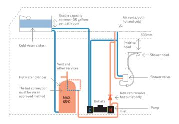
CT pump range twin ended positive head with up and over pipework and natural flow of  $1 \mbox{Litre}/\mbox{min}$  per side.
